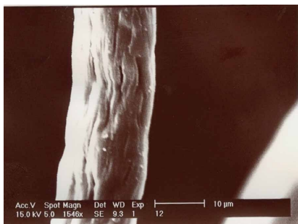
Fig. 9. SEM photograph of ungrafted PAN fibers (Magnification of 1500).
